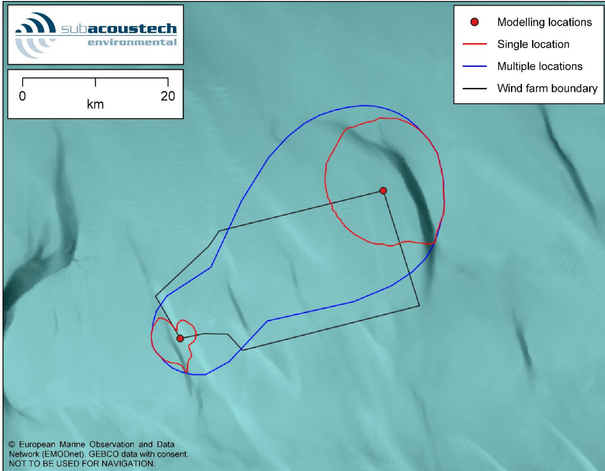
Figure 4-1 Contour plot showing the interaction between two noise sources when occurring simultaneously (TTS in fish, 186 dB SEL cum , fleeing animal)
